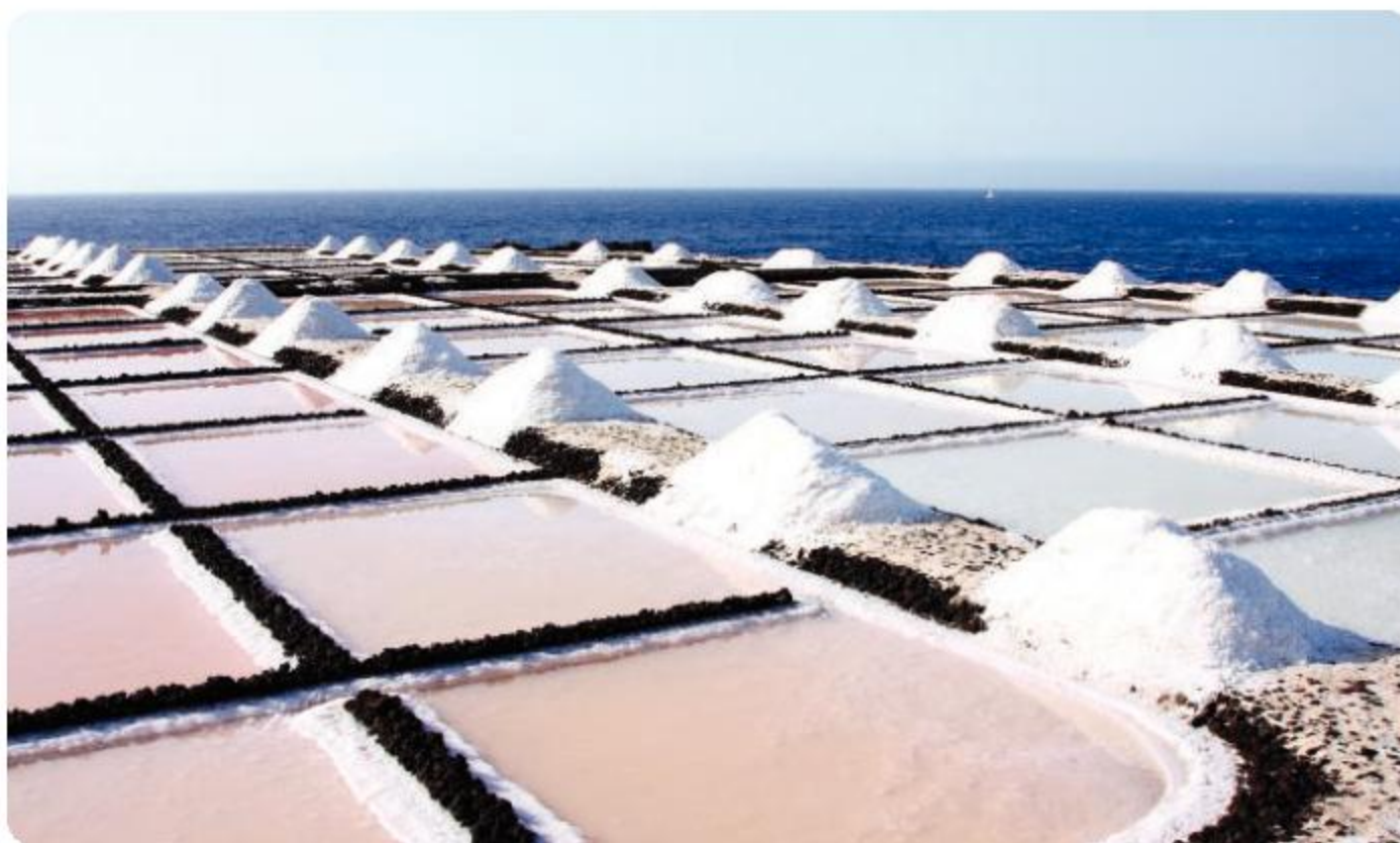
▲ Evaporation can be used to extract table salt (mostly sodium chloride) from seawater
