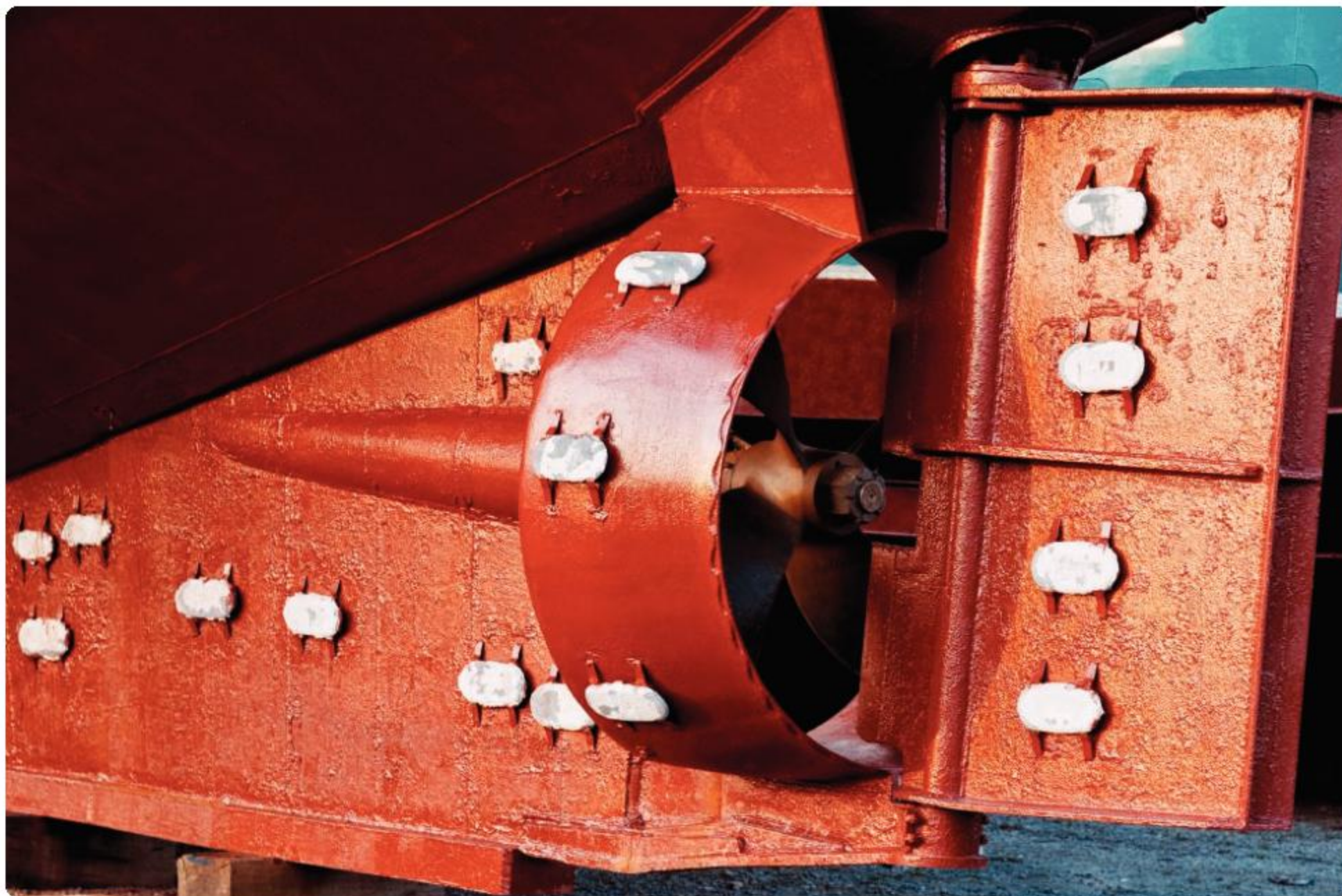
▲ Sacrificial anodes on the rudder and propeller of a fishing trawler
