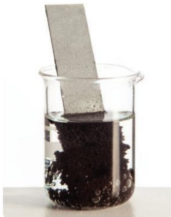
▲ Zinc metal after it has been left in copper sulfate solution
