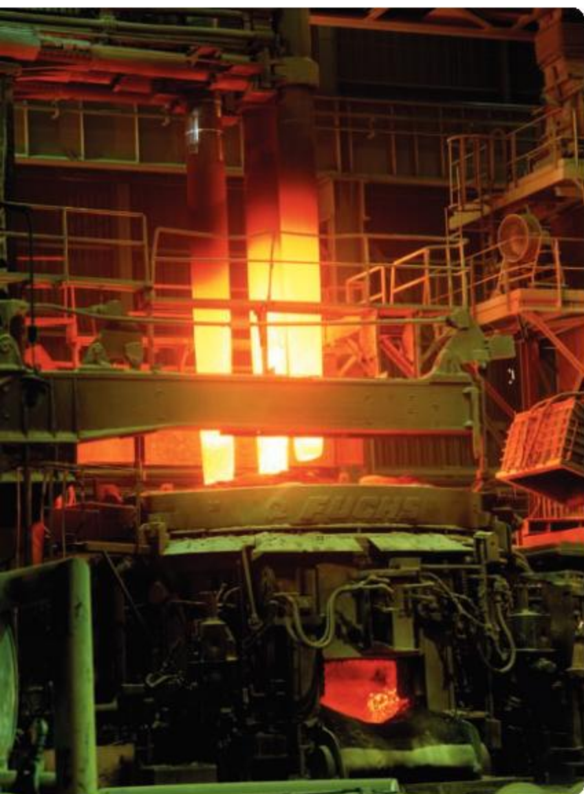
▲ Inert graphite electrodes are used in steel production
